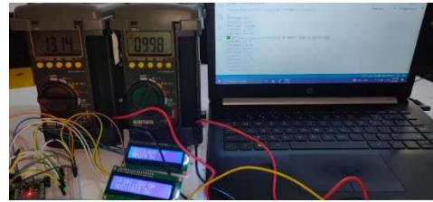
Figure 5. Smart resistivity meter system voltage output testing
