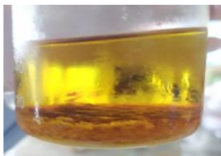
Figure 4. The process of saturating the solution with acetone: n -hexane (1:3).
