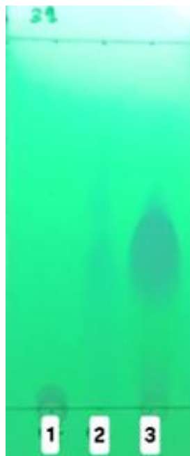
Figure 2. Thin-layer chromatography (TLC) analysis of the fraction containing citronellyl caffeate after column chromatography using n-hexane:ethyl acetate (9:1, v/v) as the solvent system. From left to right: (1) caffeic acid, (2) citronellol, and (3) citronellyl caffeate.
