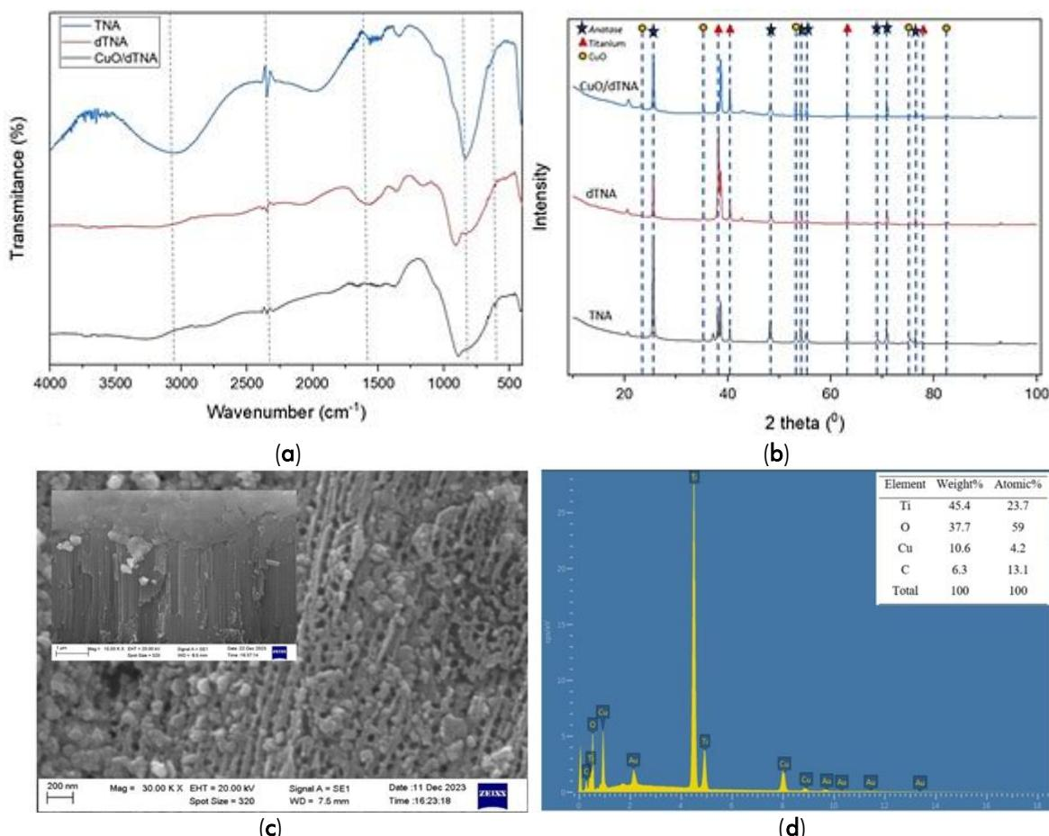
**Figure 2.** (a) FTIR characterization of TNA (blue); dTNA (red); and CuO/dTNA (black); (b) Diffractogram of TNA; dTNA; and CuO/dTNA; (c) SEM of CuO/dTNA. Inset is an enlargement of the cross-section view; (d) EDX spectra of CuO/dTNA
