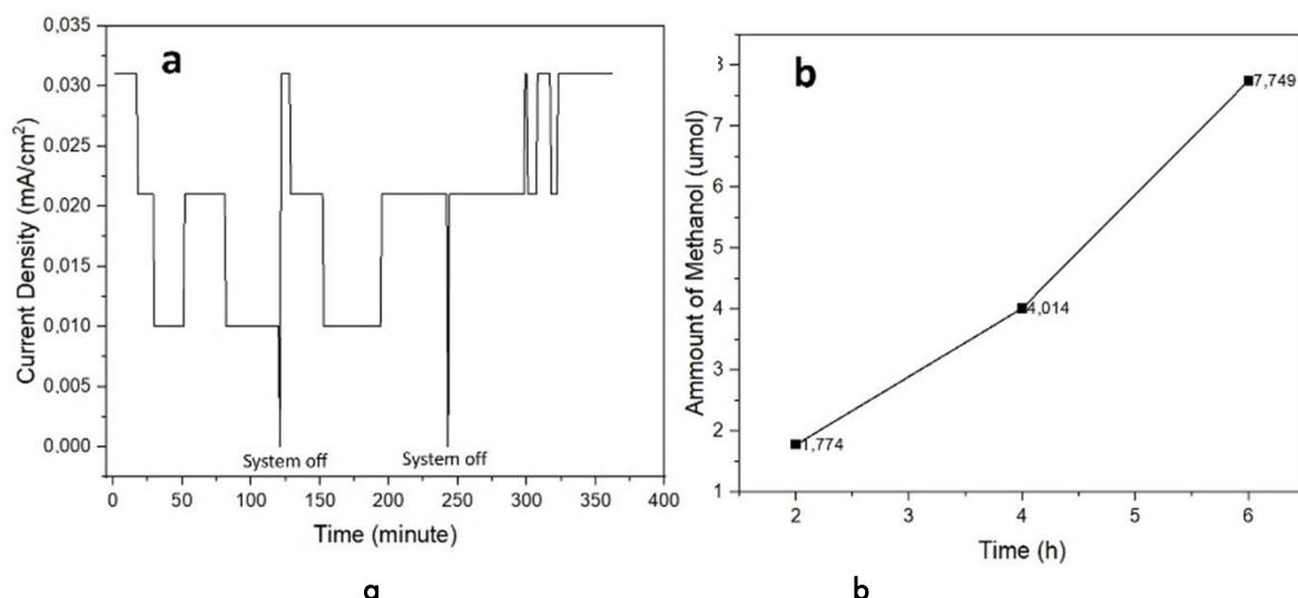
**Figure 6.** (a) The current versus time curve of CO<sub>2</sub> reduction in tandem system; and (b) Amount of methanol produced in DSSC-PEC tandem system.
