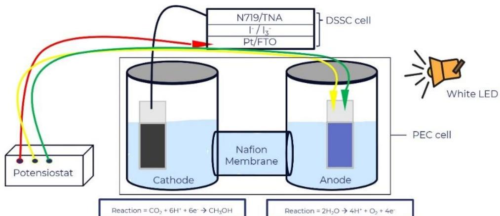
**Figure 1.** The schematic arrangement of the DSSC-PEC tandem for a photoelectrochemical  $\text{CO}_2$  reduction
