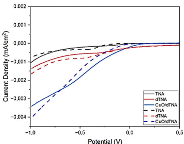
**Figure 3.** Cathodic Linear Sweep Voltammetry in electrolyte  $\text{NaHCO}_3$  pH 7 saturated  $\text{CO}_2$  (solid line) and no  $\text{CO}_2$  (dash line) with a scan rate of 20 mV/s
