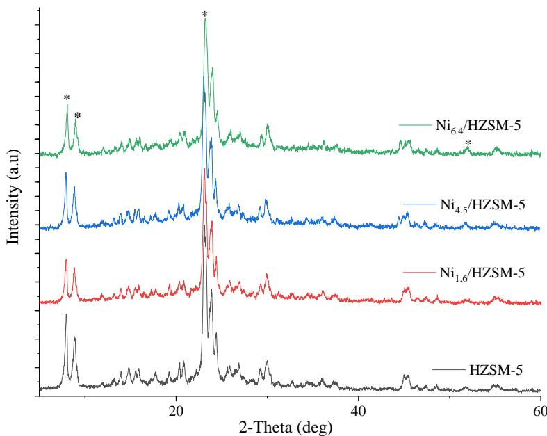
**Figure 2.** Diffraction patterns of the HZSM-5, Ni<sub>1.6</sub>/HZSM-5, Ni<sub>4.5</sub>/HZSM-5, and Ni<sub>6.4</sub>/HZSM-5.
