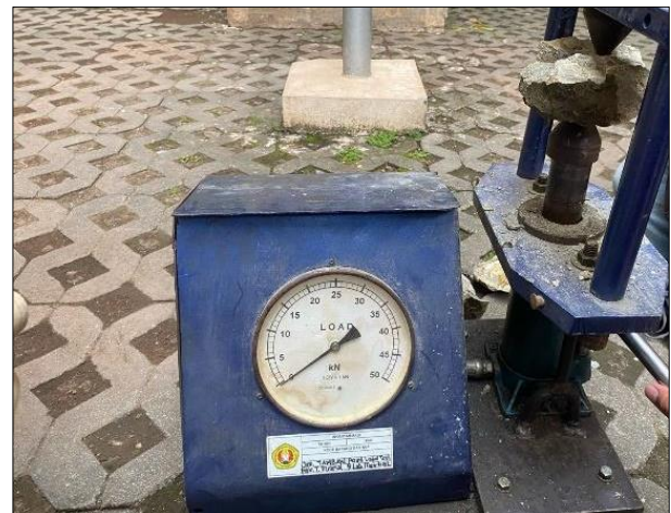
Fig. 6. Point Load Test at Rock Mechanics Laboratory.
