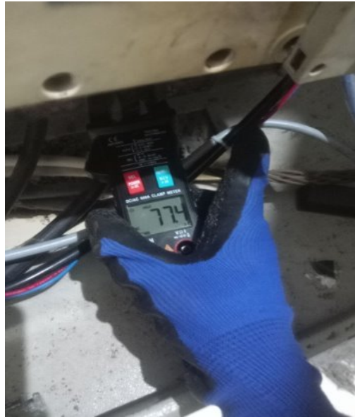
Figure 3 Manual Measurement Using Clamp Multimeter
